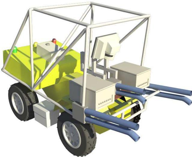
Fig. 2. The AMOR model is shown here where six blowing devices corresponding with six pipes are mounted at front of the robot.
